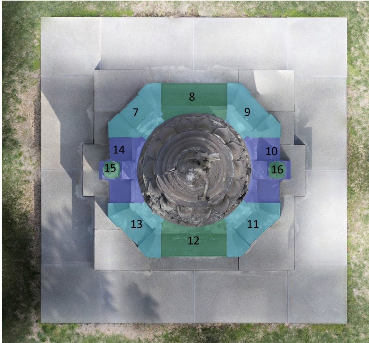
Figure 17. Confederate Memorial (000-1235). Ortho-imagery generated from photogrammetric model from HABS 2022 Study: bird's eye view. Image annotated to show major components of the octagonal bronze base.
