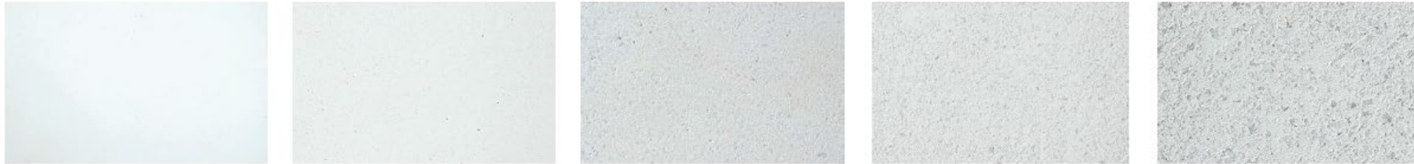
PALE PRECAST FINISHES As-cast, Sandblasted, Acid-etched, Exposed Aggregate
